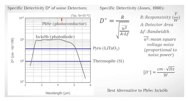
The alternatives to PbSe photoresistive detectors are thermal pyroelectrical detectors, thermal thermopile detectors and InAsSb photodiode detectors. It can clearly be seen that PbSe is technically superior to the known alternative materials (detectivity D\* almost an order of magnitude higher). So a 1:1 substitution of PbSe with another material yielding the same performance is to our present knowledge not possible.
