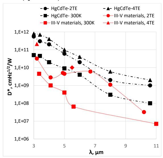
Despites years of development there are no commercially available III-V detectors that would match the performance levels of MCT detectors. Detectivity level of III-V detectors is still significantly lower than mercury-cadmium sensors – even up to 2 orders of magnitude (MCT detectors are 100x better than III-V detectors at some wavelengths, especially at LWIR spectrum).
