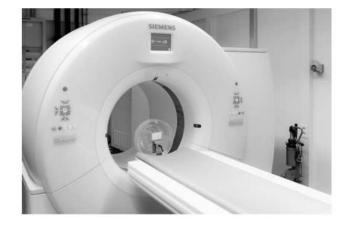
Fig.4 Hybrid CT scanner equipped with both CdTe counting detector and conventional GOS-based energy integrating detector. Fig.5 shows the optimized relative CNR<sup>2</sup> at various X-ray tube voltage. The image quality of the CdTe photon counting system increases with tube voltage. <u>The quality at tube voltage 140kV shows 46% better than the conventional detector at the same patient dose.</u>
