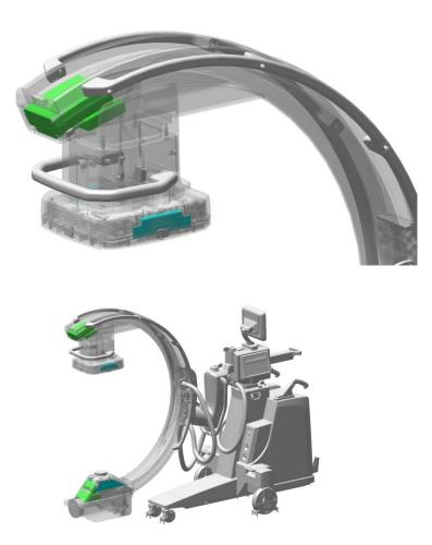
The lead counterweights need to be sizable to counter balance the weight of the C-arm and cables inside the C-arm. Due to limited space near the x-ray tube and detector the shapes have been made to fit unique shapes to make use of all available space.
