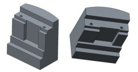
Figure 5. Couterweights used with fluoroscopy C-arm X-ray. Simple to make from lead, but much more difficult wite ungsten.
