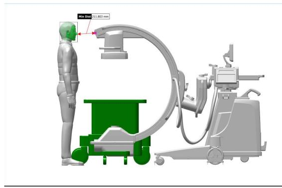
Figure 2. Surgeon standing next to patient. In this position, the gap between their head and the edge of the C-arm is 211.8mm
