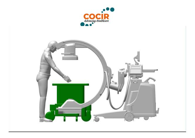
Figure 3. Theoretical position of surgeon while operating on a patient if steel counterweights are used. This is impossible as the edge of the C-arm prevents the surgeon from standing over the patient and so they would not be able to view them properly
