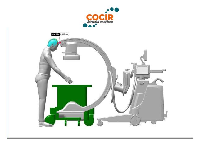
Figure 1. Position of surgeon when operating on a patient. There is a 6.4mm gap between their head and the edge of the c-arm when lead counterweights are used
