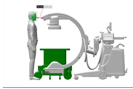
Figure 4. Surgeon standing next to patient. In this position, the gap between their head and the edge of the C-arm is 137mm.
