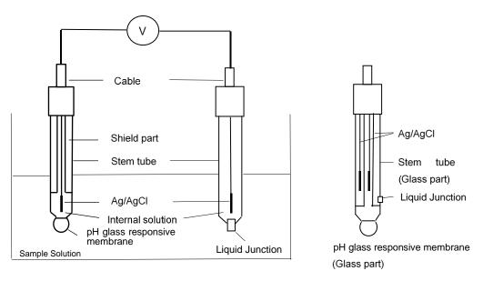
Figure.1 Configuration example of a pH electrode
