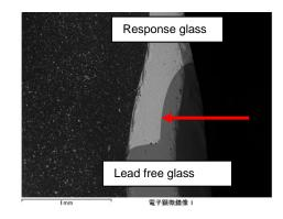
Figure 8 SEM photograph of the joint between lead free glass and pH response glass
