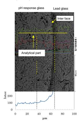
Figure 6 Analysis of lead distribution in the joint between lead glass and pH response glass
