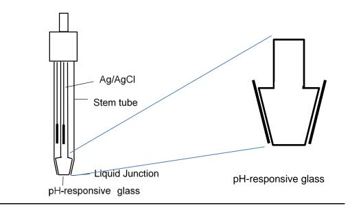
Figure. 3 Flat type example configuration
