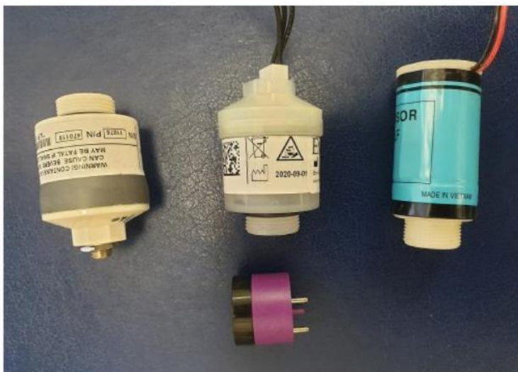
Figure 19-8: Comparison of an Alphasense O2A2 sensor and galvanic lead-free partial pressure sensors
