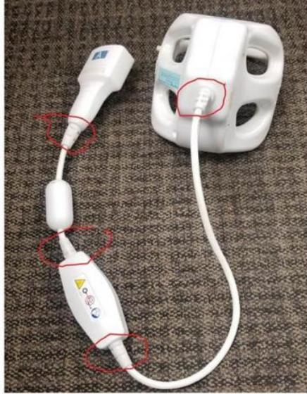
Figure 24-1: MRI shoulder coil with cable connects containing DEHP
